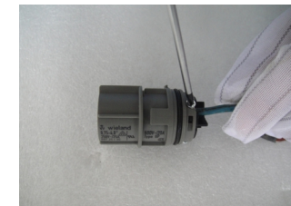
▲ Figure 4.16 Connect Wires to the Terminal
