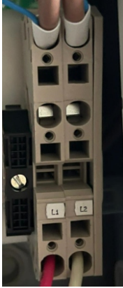
Figure 4.10 AC Connection Area of Inverter
