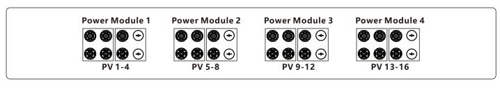
If four power modules are indeed required to connect the solar panels unevenly, for a power module which is connected to three strings, it is necessary to ensure that the power of each PV string connected under this power module does not exceed 12.2kW to achieve better power generation performance. In the case that the power difference between each PV string is less than 10%, the 3 common cases are showing below.
