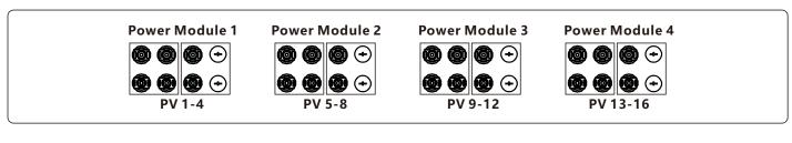
If four power modules are indeed required to connect the solar panels unevenly, for a power module which is connected to three strings, it is necessary to ensure that the power of each PV string connected under this power module does not exceed 11.3kW to achieve better power generation performance. In the case that the power difference between each PV string is less than 10%, the 3 common cases are showing below.
