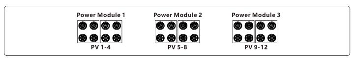
If three power modules are indeed required to connect the solar panels unevenly, for a power module which is connected to four strings, it is necessary to ensure that the power of each PV string connected under this power module does not exceed 8.5kW to achieve better power generation performance. In the case that the power difference between each PV string is less than 10%, the 2 common cases are showing below.
