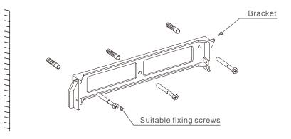
▲ Figure 4.4 Inverter wall mounting
