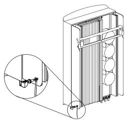
▲ Figure 4.19 Connect the external grounding conductor
