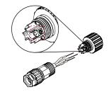
▲ Figure 4.16 Connect Wires to the Terminal
