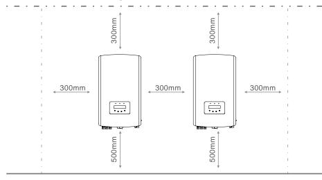
▲ Figure 4.2 Inverter Mounting clearance
