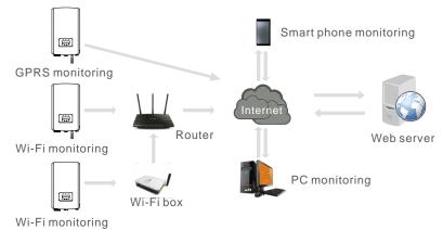
▲ Figure4.20 Wi-Fi or GPRS communication function
