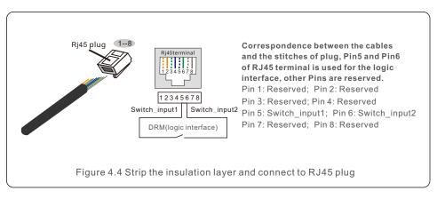
3. Connect RJ45 to DRM (logic interface).
