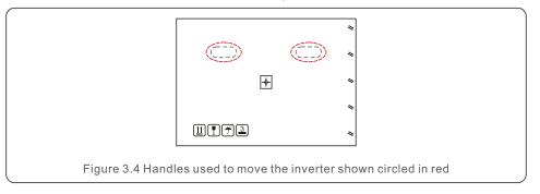
2. Two people are required to remove the inverter from the shipping box. Use the handles integrated into the heat sink to remove the inverter from the carton (see Figure 3.5).
