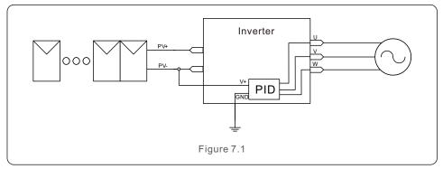
The Anti-PID module repairs the PID effect of the PV model at night. When operating, the inverter LCD screen displays "PID-repairing" information, and the red light is on. The Anti-PID function is always ON when AC is applied.
