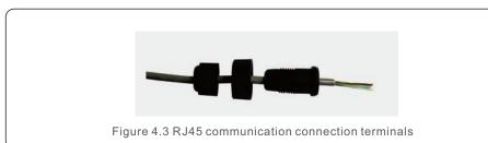
2.Use the network wire stripper to strip the insulation layer of the communication cable. According to the standard line sequence of figure 4.4 connect the wire to the plug of RJ45, and then use a network cable crimping tool to make it tight.
