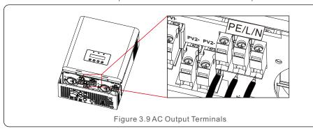
7. Ensure the wires are securely connected.
