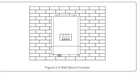
Fix the two holes on the top of the machine and one hole in the box with screws.
