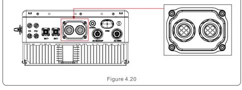
Inverter in the package is with a protective cover assembled to protect the communication ports.
