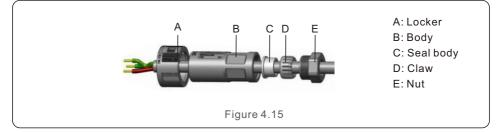
3. Crimp wires screw twisting torque 0.8+/-0.1N  $\cdot$  m.
