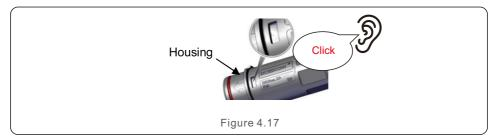
5. Insert Seal and Clamp Finger into socket ,then tighten the nut , torque 4+/-0.5N·m.
