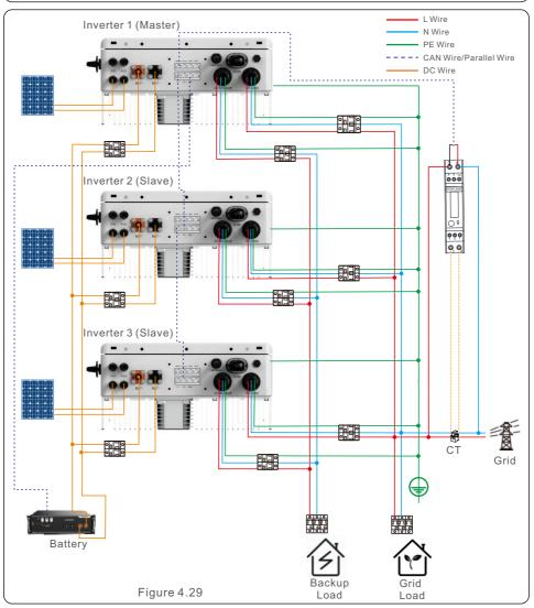
When multiple inverters are connecting in parallel, ONLY same model (same power rating) can be used.
