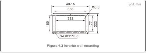
Once a suitable location has be found accordingly to 4.1 using figure 4.3 mount the wall bracket to the wall.
