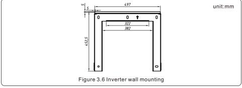
Once a suitable location has be found according to 3.1 using figure 3.6 mount the wall bracket to the wall.
