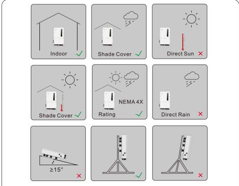
Figure 3.1 Recommended Installation locations
