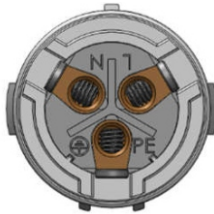
Figure 4.13 AC Grid Terminal Connector Inside
