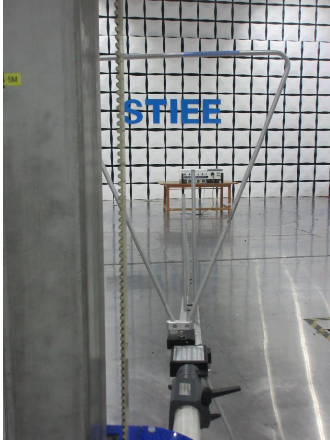
Photograph 1: Set-up for measurement of radiated emission
